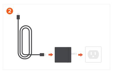
Connect the USB-C charging cable (included) to the 45W power adapter (included). Attach included wall plug adapter depending on your region. At least 36W Power Adapter required for optimal use.
