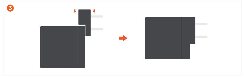
Press down until adapter sits flush with power adapter.
